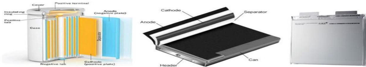
Figure 1. Li-ion cylindrical cell composition [2] Figure 2. Li-ion prismatic cell composition [3]
